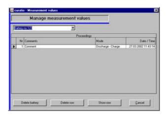
You can display and print recorded battery data using the function "Edit" and "Manage measurement values" in the window "Main Selection".
