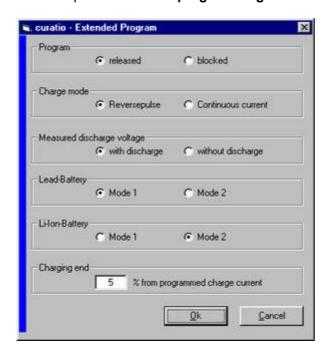
"Block programming" blocks programming via the charger keys. The charger program can only be changed via the personal computer.
