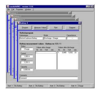
When the program "curatioWIN3" starts, the APL requests the battery program and the battery measurement values from the charger that may have already been entered, and displays them. If there is no charger connected, a message to that effect is displayed. The footer in the window "program" will show the condition of the charger channels. The charging device curatio APL-1 offers one active window, the curatio APL four windows.
