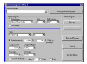
In the window "program", all parameters for discharging and charging the battery can be set and then sent to the *curatio* APL.
